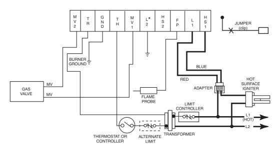
\* NOTE: Ground this terminal if model being replaced does not have 120V neutral
