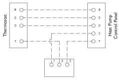
Figure A: Geothermal Zone Valve Wiring to a Heat Pump Control
