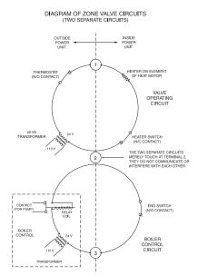
Figure C: Zone Valve Circuits
