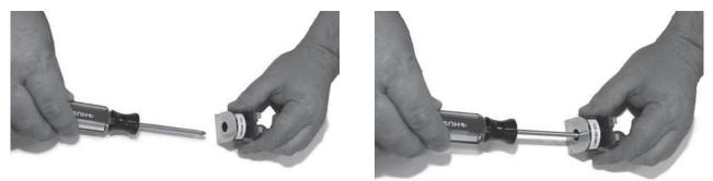
To check the solenoid's magnetic pull, begin by pulling solenoid off of reversing valve. Then energize solenoid and place a metal screw driver in solenoid. You should feel the screw driver being pulled by the magnetic field.
