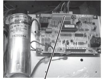
2) Remove this Molex plug to check resistance of the FP1/ LT1 sensor
