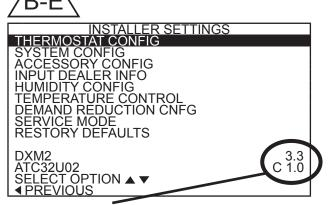
Locate the version level of the DXM2 board and thermostat or service tool on the screen. You can locate the part number on the board and compare it to the table below.
