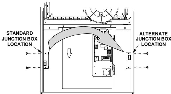
**90% Furnace Junction Box Relocation**
