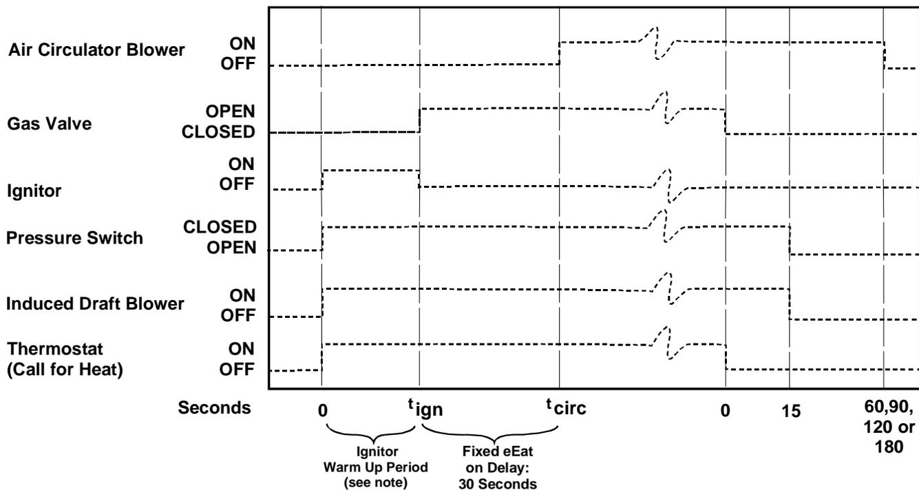
NOTE: **HEATCRAFT** INTEGRATED CONTROL MODULE HAS A FIXED STANDARD SEVEN-SECOND IGNITER WARM UP PERIOD (MINI IGNITER).
