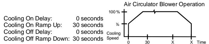
**NOTE:** This option of no cooling "ON" or "OFF" air circulator blower delay is only available on GUIV-CA/DX & GUAV-AX models.
