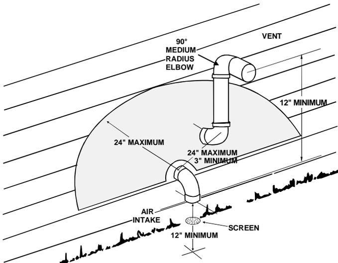
**90% Furnace Alternate Horizontal Vent Termination (Dual Pipe)**
