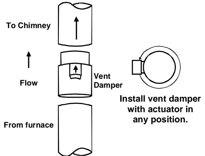
Install vent damper with actuator in any position.
