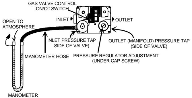
**Measuring Inlet Gas Pressure (Gas Valve Tap)**
