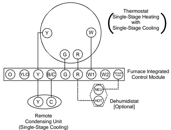
NOTE: To apply a single-stage heating thermostat, the thermostat selector jumper on the integrated control module *must* be set on single stage.
