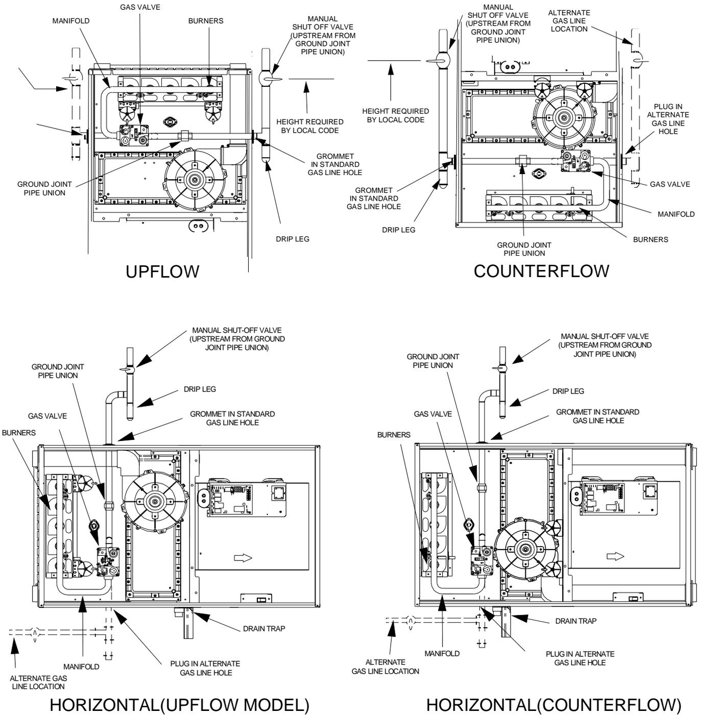
NOTES: 1. WHEN GAS LINE IS IN THE ALTERNATE LOCATION, SWAP THE POSITION OF THE PLUG AND GROMMET.
