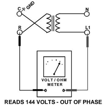
If meter reads approximately 96 volts - the primary to secondary are in phase - if reads approximately 144 volts out of phase - reverse low voltage wires.
