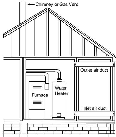
\*If the appliance room is located against an outside wall and the air openings communicate directly with the outdoors, each opening shall have a free area of not less than one square inch per 4,000 BTU per hour of the total input rating of all appliances in the enclosure.
