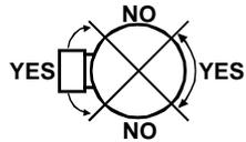
Install vent damper with actuator to sides of vent only. Do not mount vent damper with actuator above or below the vent.
