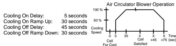
If "Y" from the thermostat is connected to "Y/Y2" on the air circulation motor interface board, then the following on and off sequences will occur.
