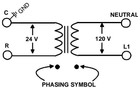
Some transformers will display phasing symbols as shown in the illustration to the left to assist in determining proper transformer phasing.
