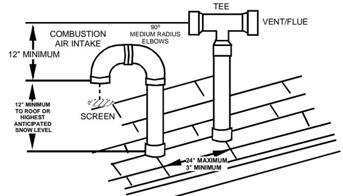
90% Furnace Vertical Terminations (Dual Pipe)
