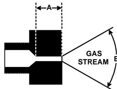
The length of Dimension "A" determines the angle of Gas Stream "B".
