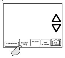
Upon entering the advanced menus, the Advanced Fault Menu is displayed. The display will change to the Fault Screen and indicate any faults that may be present in the indoor or outdoor equipment. If a fault is present, the Fault Screen will show the equipment and an error code with a description of the fault. Touch do not be keys to view the fault status of any remaining equipment. The text "NO FAULTS" will be scrolled if no errors are
