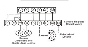
Thermostat - Two-Stage Heating with Single-Stage Cooling
