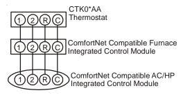
**System Wiring using Four-Wires**
