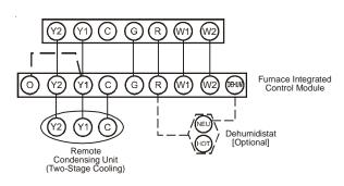
Thermostat - Two-Stage Heating with Two-Stage Cooling
