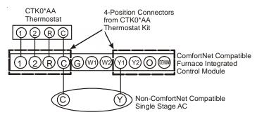
System Wiring between Furnace and Non-Communicating Compatible Single Stage Air Conditioner
