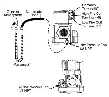
Honeywell Model VR9205 Connected to Manometer
