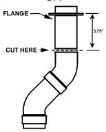
Vent/Flue Pipe Cuts
