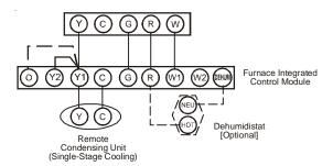
**NOTE:** To apply a single-stage Heating Thermostat, the thermostat selector switch on the Integrated Control Module *must* be set on single-stage.
