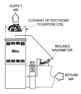
**Checking Static Pressure** (80% Furnace Shown, 90% Similar)
