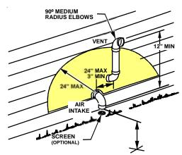
Alternate Horizontal Vent Termination (Dual Pipe)
