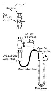
Measuring Inlet Gas Pressure (Alt. Method)
