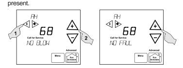
Touch the ♠ or ▶ to step through the list of installed equipment, including the thermostat. Touch the **Installer Config** key to enter the submenus for the equipment displayed. The text "**WORKING**" will be displayed in the scrolling display area while the data is being retrieved. The first sub-menu is then displayed. See tables below for listing of furnace submenus.
