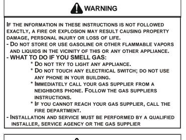
SHOULD OVERHEATING OCCUR OR THE GAS SUPPLY FAIL TO SHUT OFF, TURN OFF THE MANUAL GAS SHUTOFF VALVE EXTERNAL TO THE FURNACE BEFORE TURNING OFF THE ELECTRICAL SUPPLY.
