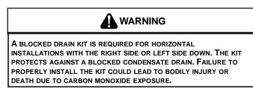
**NOTE:** This furnace is shipped from the factory as a Dedicated Upflow. A "Blocked Drain Kit" is available and <u>MUST BE USED</u> if the furnace is installed Horizontal Left or Horizontal Right. Check the Serial/ Rating Plate on the furnace for the Kit P/N.
