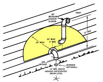
**Alternate Horizontal Vent Termination (Dual Pipe)**
