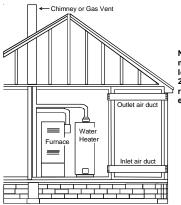
NOTE: The air duct openings must have a free area of not less than one square inch per 2000 BTU of the total input rating of all equipment in the enclosure\*.
