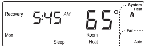
Fig. 3. Example of “Recovery” indication.
