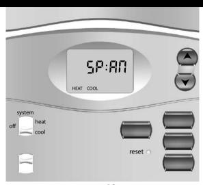
2. Span setting mode – allows you to adjust the system ON/OFF cycle rate. The default setting is 2 (the system cycles ON or OFF when the temperature is within 1° F (0.5° C) above and below the set temperature). The span setting can be adjusted if your system is cycling too fast or too slowly.
