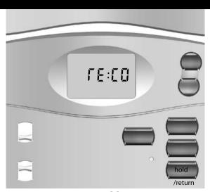
4. Auto recovery – allows heating and cooling systems to gradually recover from an energy-saving setpoint temperature to a comfort setpoint temperature. Auto recovery calculates the time needed to adjust the temperature to the next program setting. When the thermostat is in Auto Recovery mode, the display will flash alternating messages of RECO and the time. Auto Recovery can be disabled by sliding the recovery switch on the back of the circuit board to the disable position.
