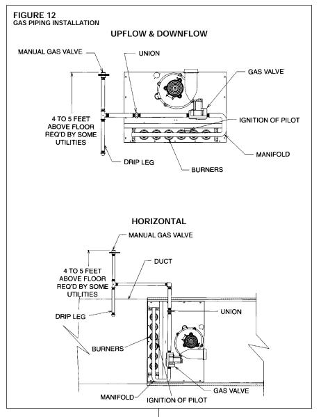
a piece of black pipe. If local codes allow the use of a flexible gas appliance connector, always use a new listed connector. Do not use a connector which has previously serviced another gas appliance. Massachusetts law limits flexible gas connectors to a maximum of 36".
