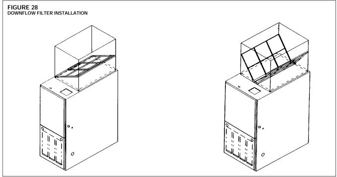
IMPORTANT: Do not operate the system for extended periods without filters. A portion of the dust entrained in the air may temporarily lodge in the air duct runs and at the supply registers. Any recirculated dust particles will be heated and charred by contact with the furnace heat exchanger. This residue will soil ceilings, walls, drapes, carpets, and other household articles.
