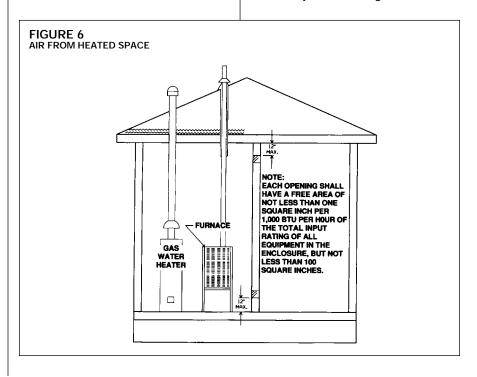
Combustion air must be free of acid forming chemicals; such as sulphur, fluorine and chlorine. These elements are found in aerosol sprays, detergents, bleaches, cleaning solvents, air fresheners, paint and varnish removers, refrigerants and many other commercial and household products. Vapors from these products when burned in a gas flame form acid compounds. The acid compounds increase the dew point temperature of the flue products and are highly corrosive after they condense.
