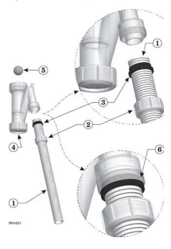
Figure 48 Condensate trap assembly into jacket
